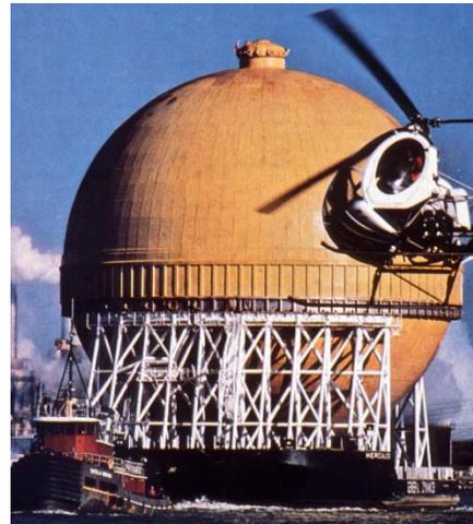
Unstiffened spherical shell for LNG tanker
