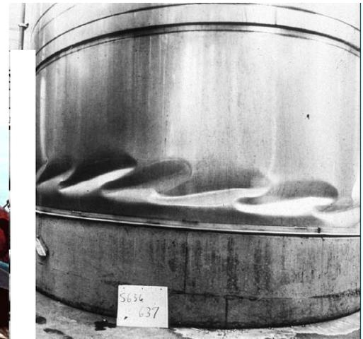
Buckled huge steel wine barrel in CA failed during earthquake
