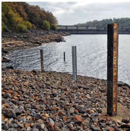
Left Depth gauges at Thruscross Reservoir, UK. Photo by Tom Blackwell via Flickr, used under CC BY NC 2.0.
