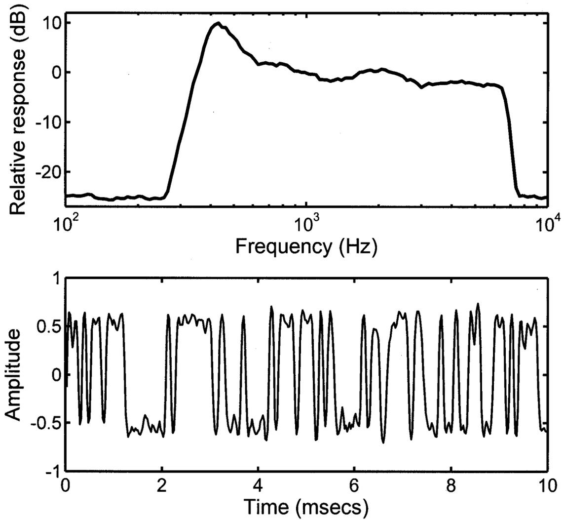
Figure 5. Showing the spectrum (top) and a segment of the waveform (bottom) of the TEN.
