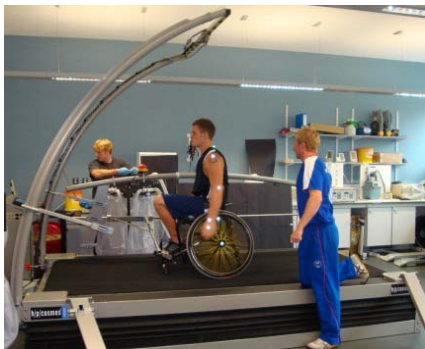
Photograph 5: A participant performing a trial on the treadmill with joint markers on for video analysis.
