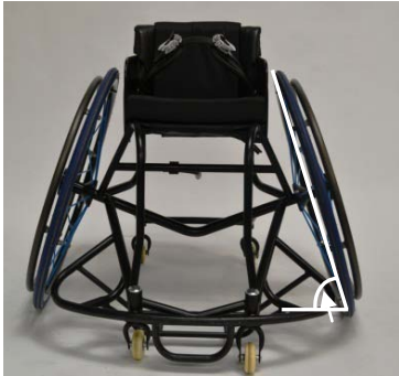
Photograph 4: A typical court sport wheelchair with rear-wheel camber
