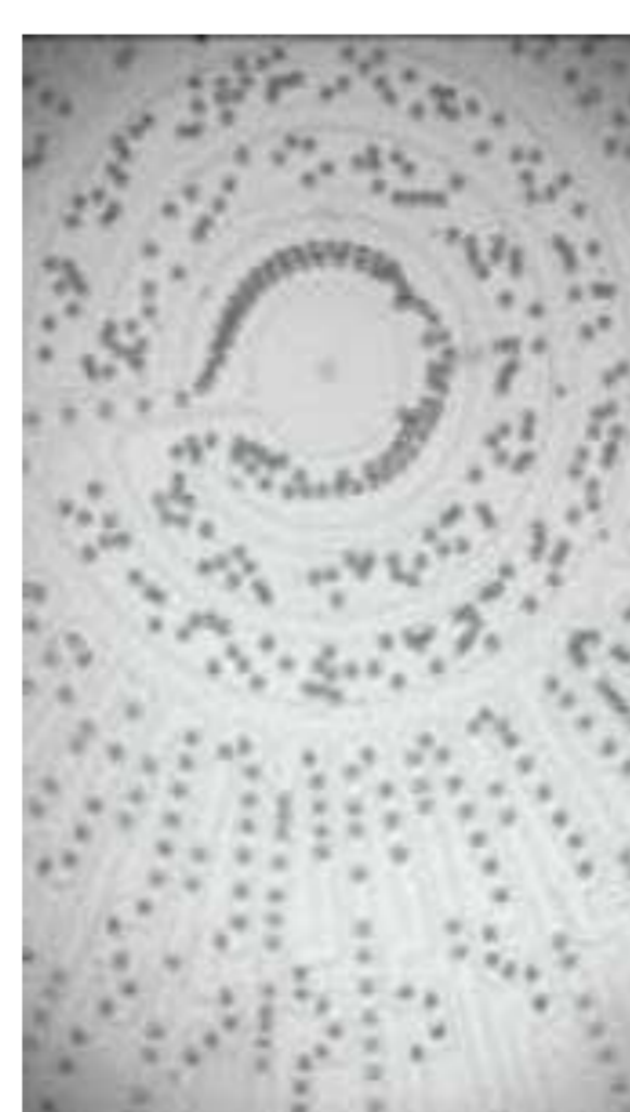
Picodroplets being moved around via an oil stream in microfluidic channels
