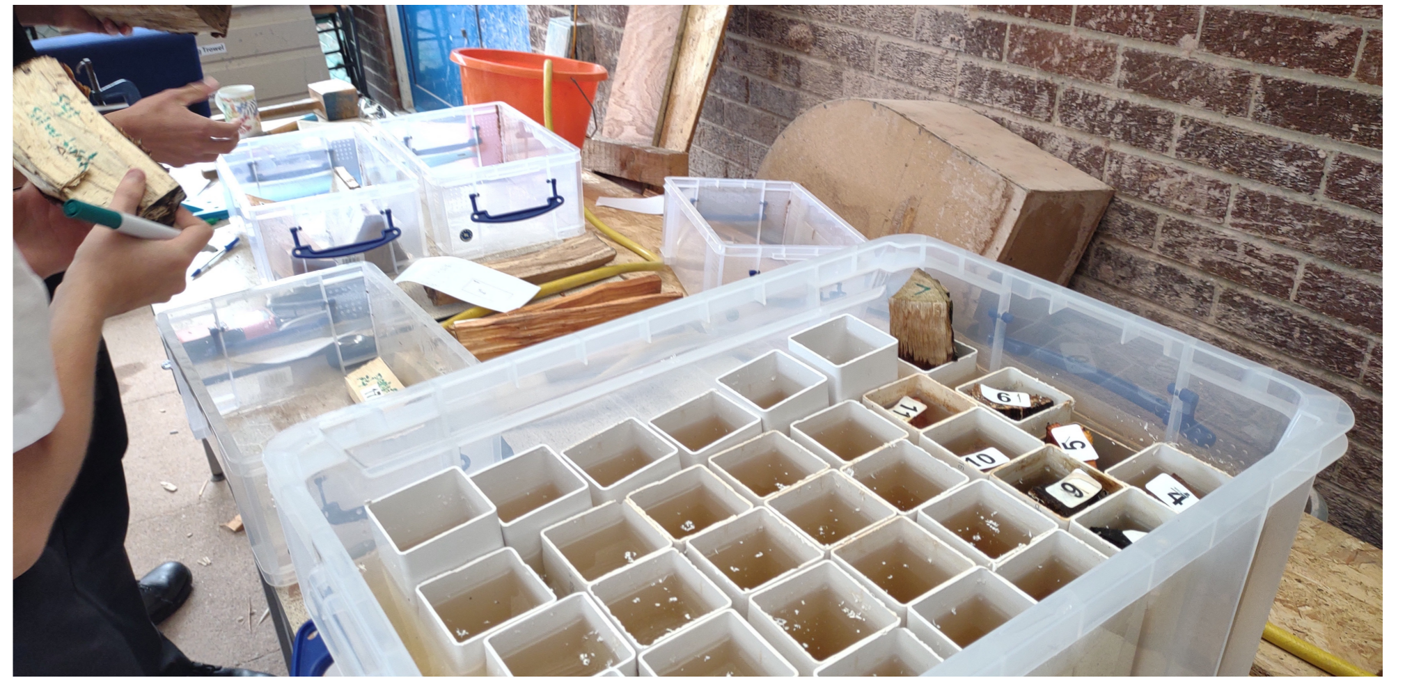
All the samples absorbed water. We measured the mass daily to work out the least absorbent.
