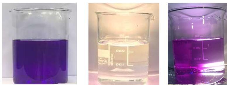
Photos showing the thionine solution before (*left*) and after (*middle*) irradiation. Two toned solution produced when half of lamp is covered (*right*).
