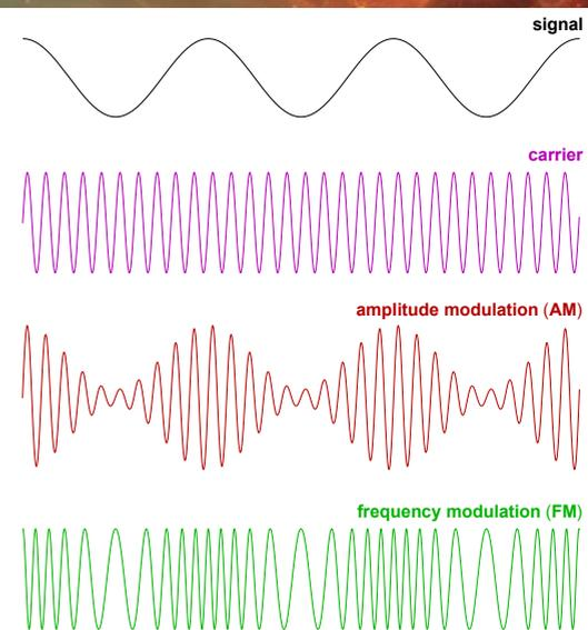
Amplitude and frequency modulation of a carrier wave by a signal.
