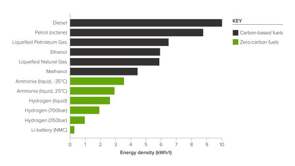
The volumetric energy density of a range of fuel options<sup>6</sup>.
