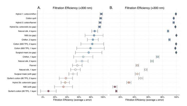
Source: Adapted from Table 1<sup>154</sup>. Note: The figure shows filtration efficiencies at a flow rate of 1.2 CFM.
