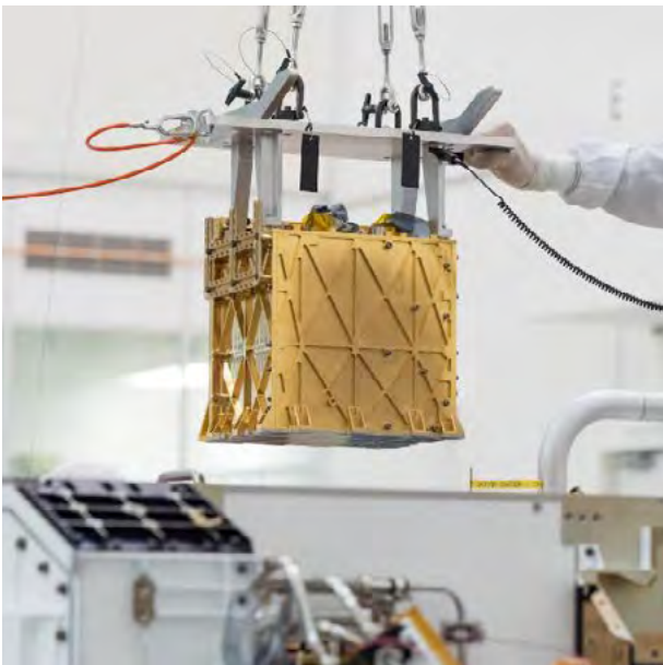
Left MOXIE (Mars Oxygen In-Situ Resource Utilization Experiment) was launched aboard NASA's Perseverance rover to test a technology for extracting oxygen from the Red Planet's carbon dioxide-rich atmosphere. © NASA/JPL-Caltech/CNES/IRAP.
