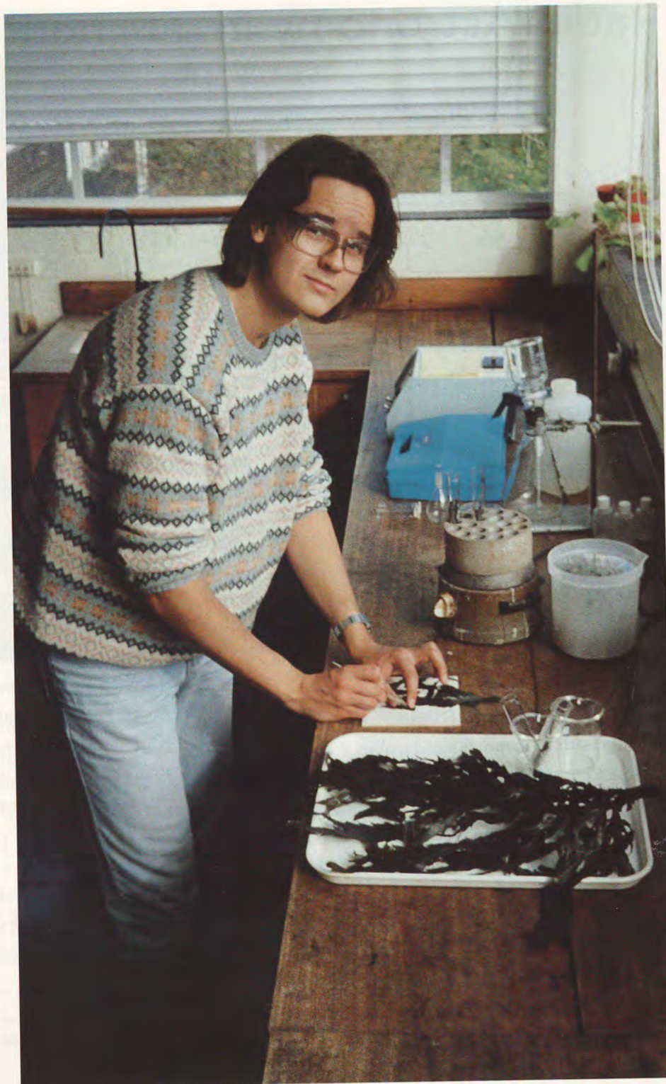
Samples of Fucus serratus are cut up prior to digestion in concentrated nitric acid.
