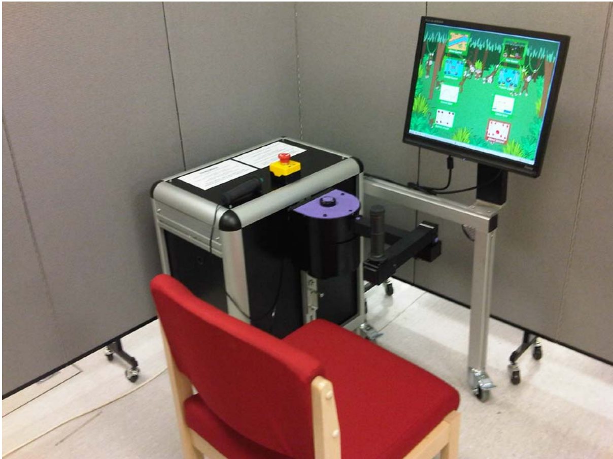
Figure 3: Single-player Assisted Movement Device for therapeutic play
