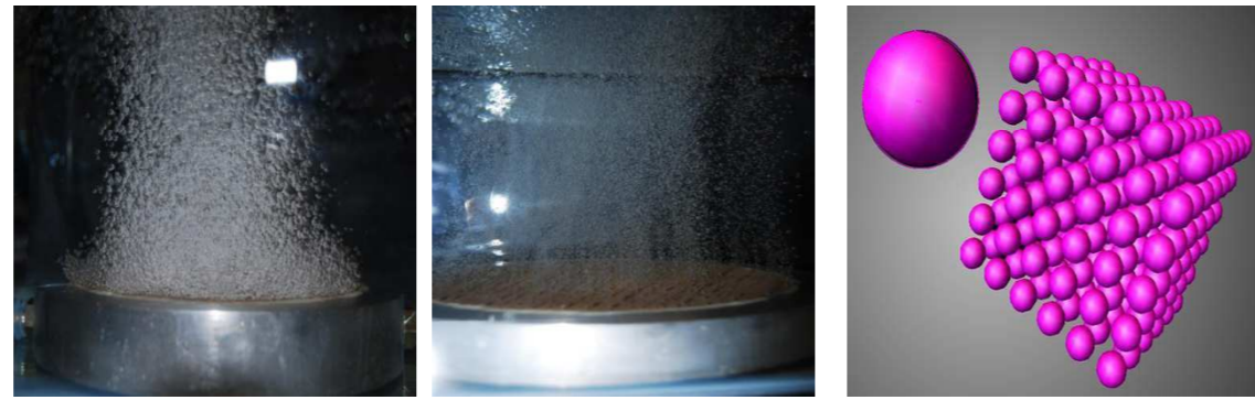
Fig. 2: Microbubbles with membrane only (a) and with membrane and oscillator (b). Comparative size of bubbles (c).
