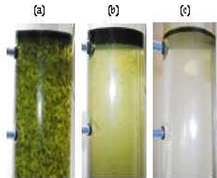
Fig. 3: Microflotation stages of clarification: (a) Flocculated algae; (b) blanket formation; (c) completed separation.
